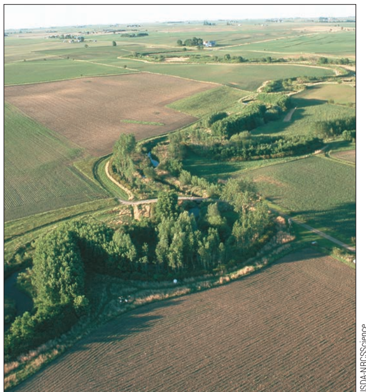
Riparian and grassed buffers can stabilize streambanks and intercept P in runoff in many situations.
